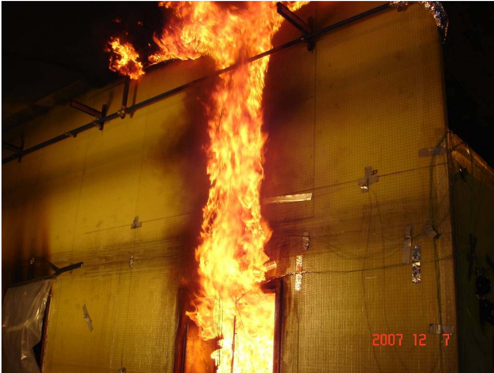
Figure 4-18 Fire spread on the outer wall from the pool fire without drencher activation.
