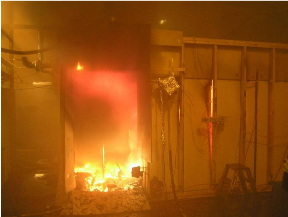
Figure 4-16 A representative photo that gives some indication of the intense heat evolved and the very high intensity of this fire. Note the separation of wall elements in the cabin (no outer bulkhead construction on this side).
