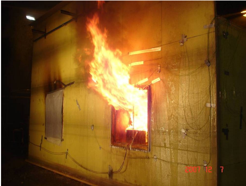
Figure 4-17 Heptane pool fire in the cabin window opening with drencher in function. The outer wall is sufficiently cooled down by the drencher and virtually no flames are seen on the outside laminate.
