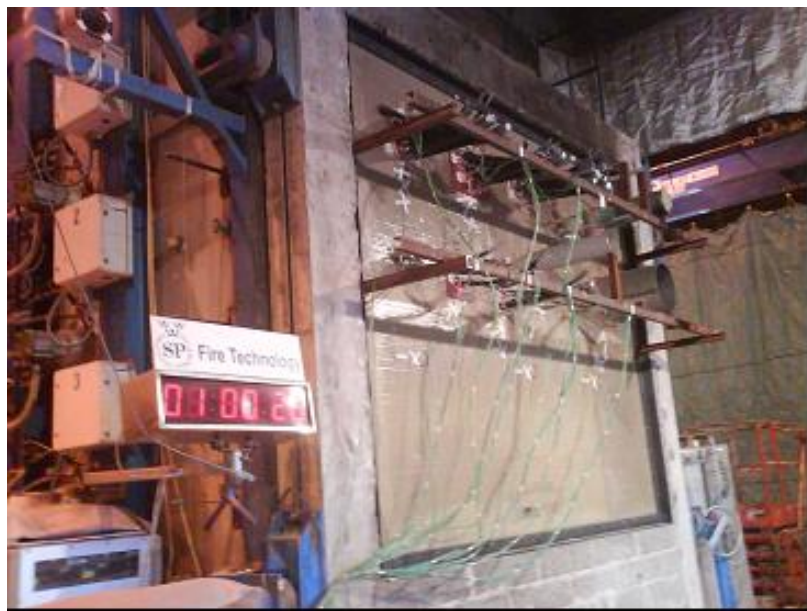
Figure 14-6 Fire resistance test performed at SP (Sweden) of bulkhead with cable, pipe and AC duct penetrations
