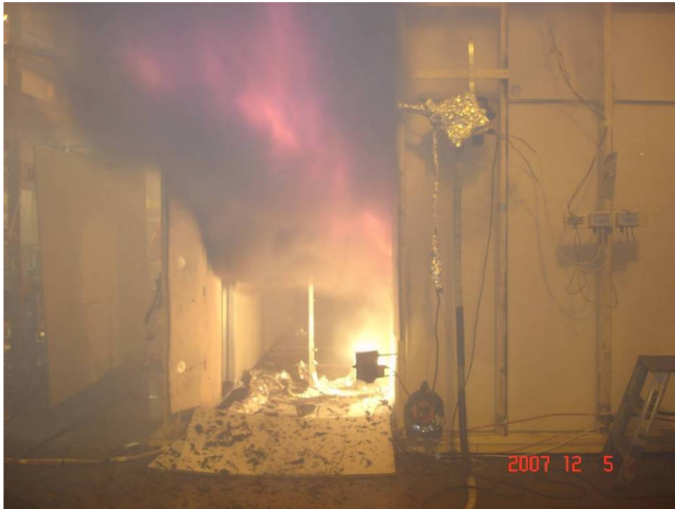
Figure 4-15 Flashover fire test. The flames emerge into the corridor from the burning cabin to the right.
