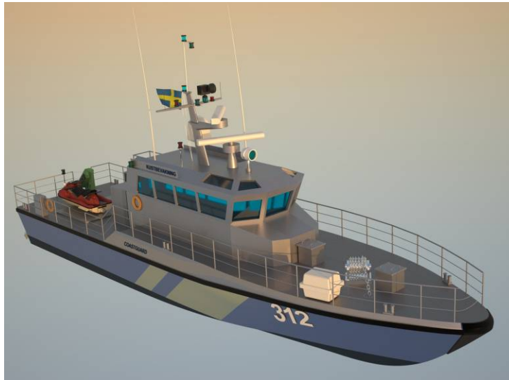
Figure 7-8 Projected new coast guard craft with composite material hull
