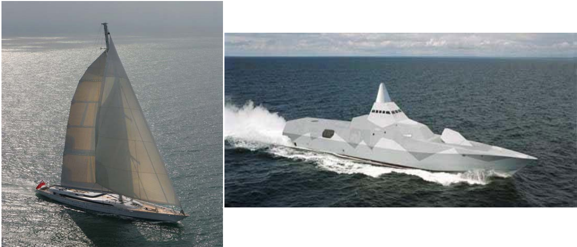
Figure 8-1 75.2 m Mirabella V and 73 m Visby Corvette - Longest Glass and Carbon Fibre vessels
