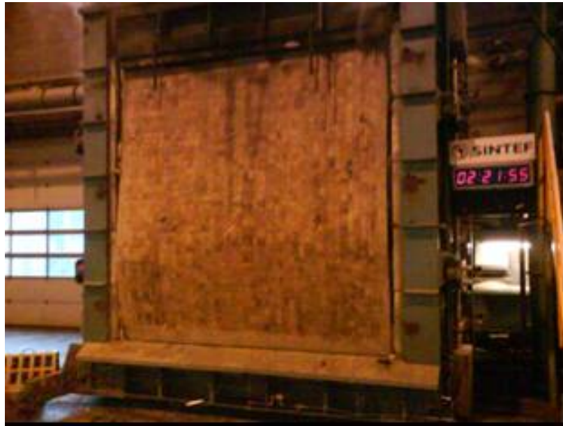
Figure 14-5 Fire resistance test performed at Sintef (Norway) of a balsa-cored bulkhead that survived 2 h 20 min
