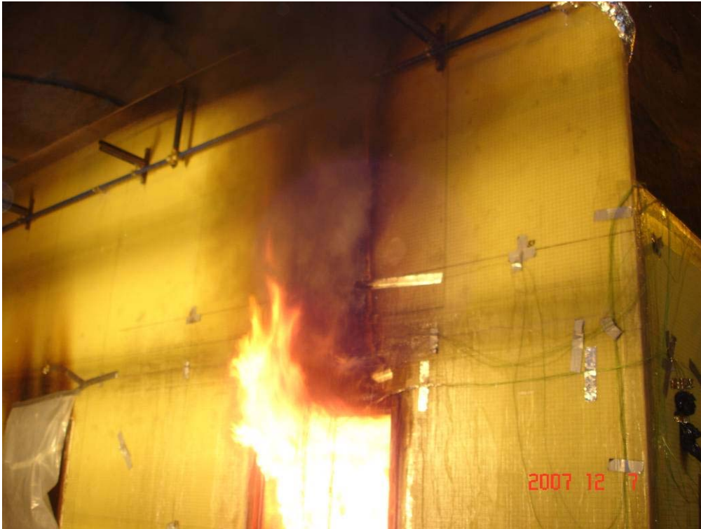
Figure 4-19 The composite outer wall a few seconds (5-10 seconds) after the drencher was activated
