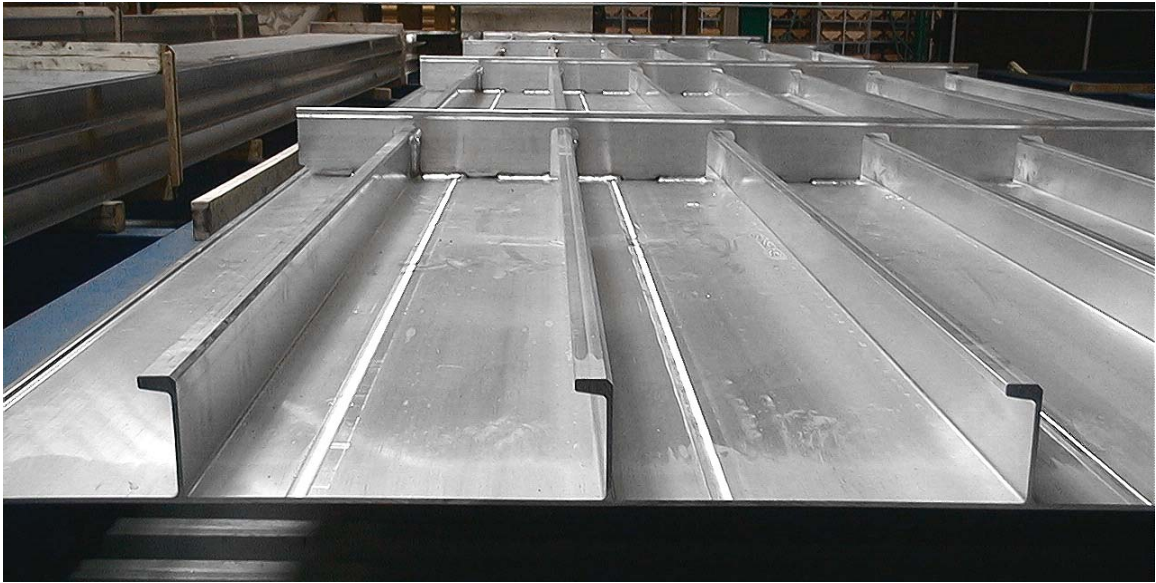
Figure 5-4 Prefabricated FSW panel with transverse stiffeners
