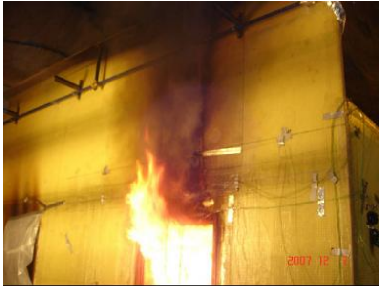
Figure 14-7 Full scale fire test trial performed at SP (Sweden) demonstrating the efficiency of a drencher system in preventing external fire propagation when an internal fire exits through a broken window
