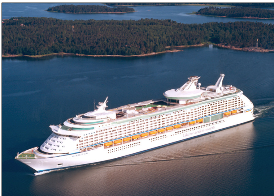
Figure 5-1 Cruise vessel with top decks made of aluminium extrusions
