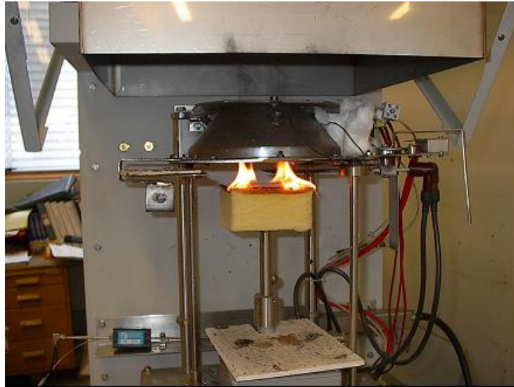
Figure 14-3 Small scale tests performed at SP (Sweden) to provide inputs to fire simulations
