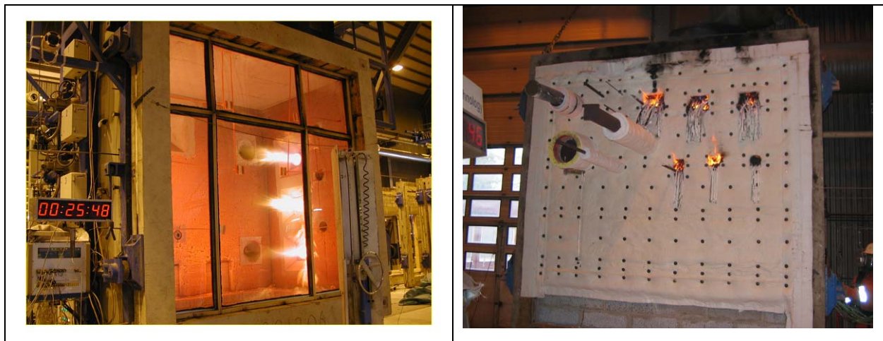
Figure 4-3 Large furnace used for bulkhead test (left) and fire exposed side of a sandwich composite bulkhead construction after successful bulkhead penetration tests in the furnace (right)
